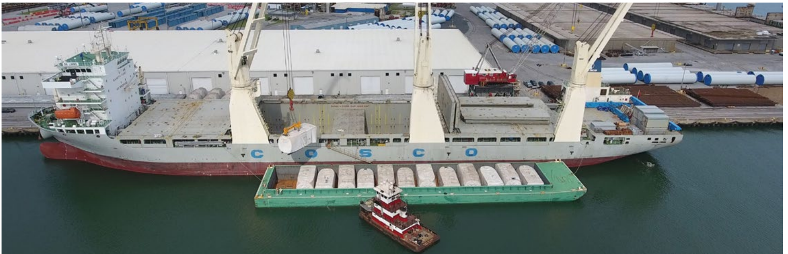
Tug and Barge receiving Wind Turbine Nacelles directly from ship's side in Morehead City NC. Amazon's Desert Wind Project
